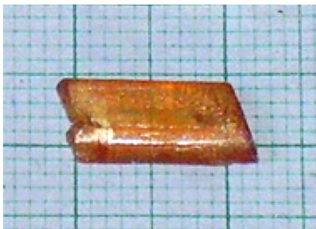
Fig. 1 As grown crystal of SPHA
